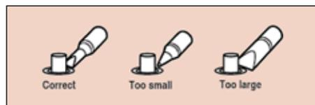
Fig. 1: Selecting the right soldering tip
